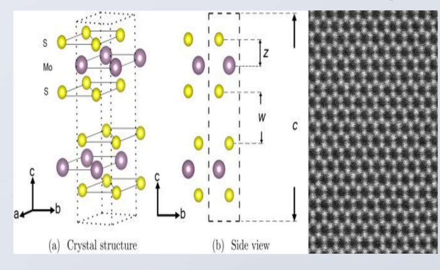
2H MoS<sub>2</sub> nanosheet imaged at 80kV, Mo and S atoms are clearly resolved.
