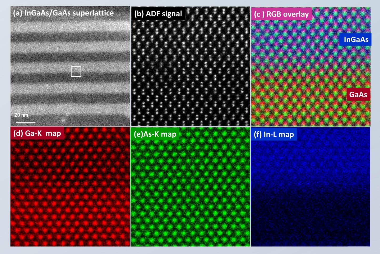
Atomic-scale elemental mapping of the interface between InGaaAs and GaAs. (a) STEM image of InGaAs/GaAs superlattice and (b) atom-resolved image showing the survey area. (c) Color-overlaid
