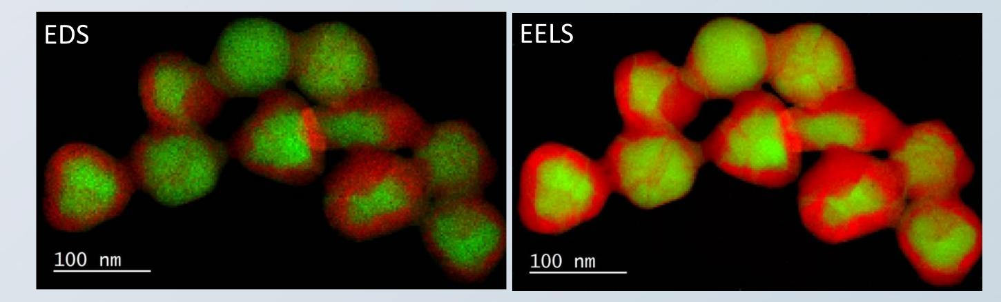
Elemental maps of Pd - Au catalyst nanoparticles (Pd in red and Au in green) acquired using EDS and
